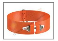
The Hinged Bolted Stop Collar is available in 4 1/2 " to 20 " sizes. It is a single piece collar and the set crews are provided on the outer circle of the periphery which is meant for installing and is directly installed on the pipe by slipping on the casing without any hassle. It is fabricated using ductile iron therefore it has a good impact and fatigue capability.
